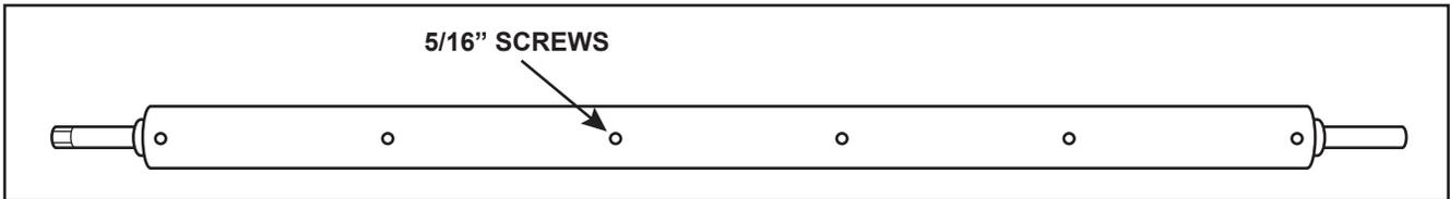
**NOTE:** If the tube assembly is damaged, you can remove it from the arms at this time. It may be necessary to loosen the ratchet strap and remove the 5/16 bolt from one end of the tracking bar to allow one arm to be moved out to make it easier.
