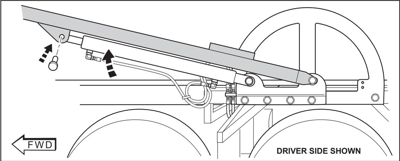
i. Install upper pivot of the Arm Extend/Retract cylinder with 1/2" x 2" Clevis Pin.
