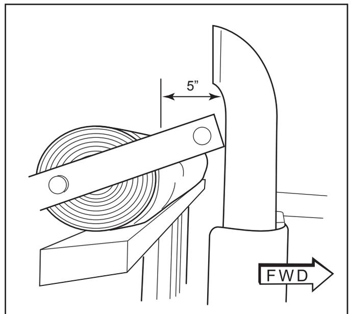
e. Fabricate brackets for Driver Side and Passenger Side as needed to fit. Notch around existing hardware or utilize existing fasteners locations if possible.
