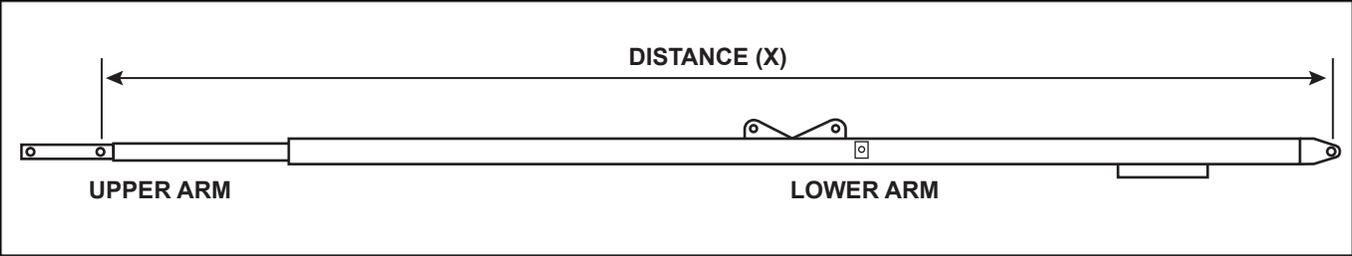
d. Pin the Arm Extension Cylinder in position on the arm and use this to determine the location of the upper arm mounting plates. **NOTE:** Be sure the cylinder piston is fully seated.
