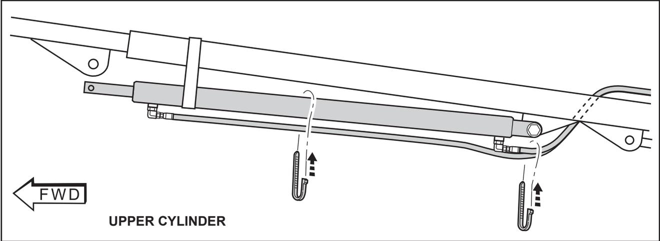
**IMPORTANT:** Bleed the system at this time to test that cylinders are operating properly.
