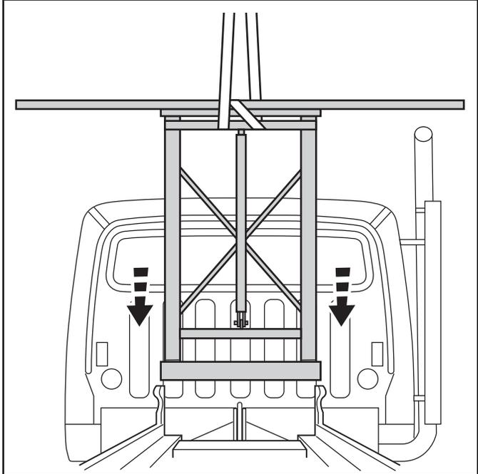
**IMPORTANT:** Check all position measurements to be sure gantry is centered, square with frame and proper clearances are all accounted for.
