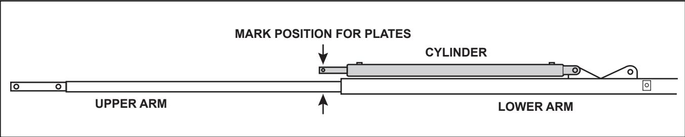
e. Clamp upper mounting plates into place using the cylinder as a guide. Weld two new cylinder mount plates onto upper arm.
