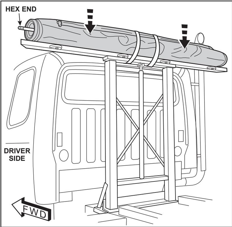
**NOTE:** Visually align the torsion axle with the center of the gantry front to back.
