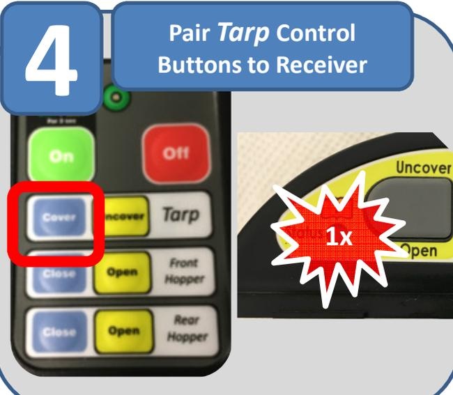
The image shows a transmitter keypad with several buttons. The 'Cover' button is highlighted with a red box. To the right, a tarp motor is shown with a red starburst containing '1x' next to the 'Uncover' button.
