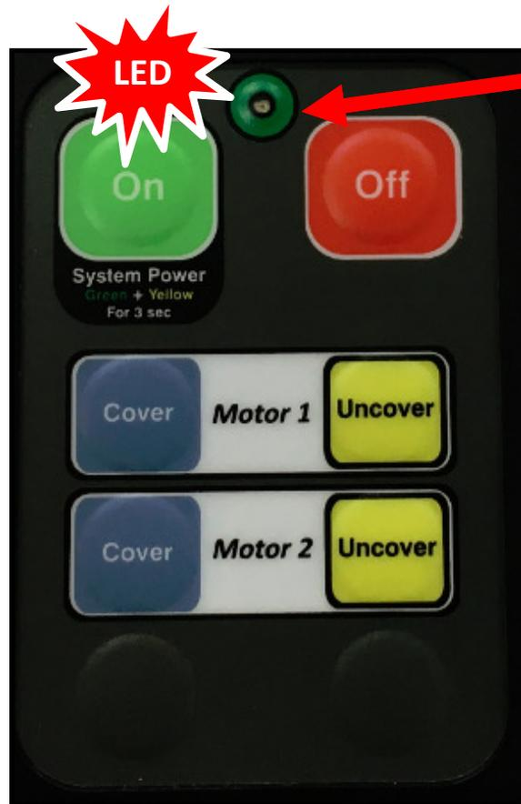
When the transmitter is operating, the **RED LED** flashes rapidly when a button is pressed. *This Indicates that communication is working between the transmitter and receiver.*
