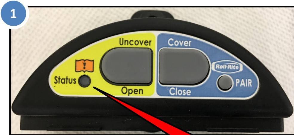
1. Make Sure the Receiver is **NOT in LOCK OUT mode** see "Locking Out Tarp System Receiver"
