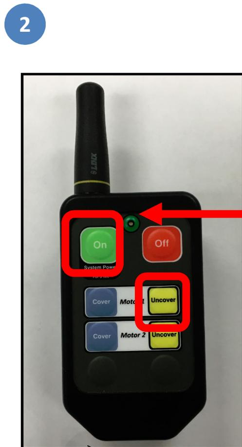
3 5X Flash Indicates Receiver and Transmitter are Both Ready to Operate System
