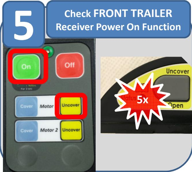
The image shows the transmitter control panel. The 'On' (green) and 'Uncover' (yellow) buttons are highlighted with red boxes. To the right, a close-up of the 'Uncover' button is shown with a red starburst containing '5x' overlaid on it.
