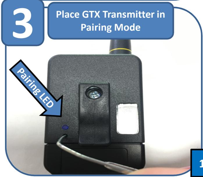
**3** Place GTX Transmitter in Pairing Mode
