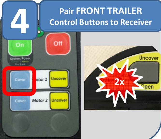
The image shows a transmitter control panel with several buttons: 'On' (green), 'Off' (red), 'Cover' (blue), 'Uncover' (yellow), and 'Motor 1'/'Motor 2' (white). The 'Cover' buttons are highlighted with a red box. To the right, a close-up of the 'Uncover' button is shown with a red starburst containing '2x' overlaid on it.
